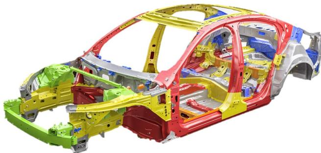
*Figure 5. Different materials, indicated by different colours, selected to maintain the structural integrity, and absorb energy. [source: Volvo Cars]*
