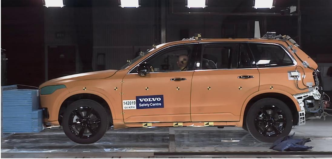
*Figure 8. A photo of a car at barrier contact; an example of a standardised crash test. [source: Volvo Cars]*
