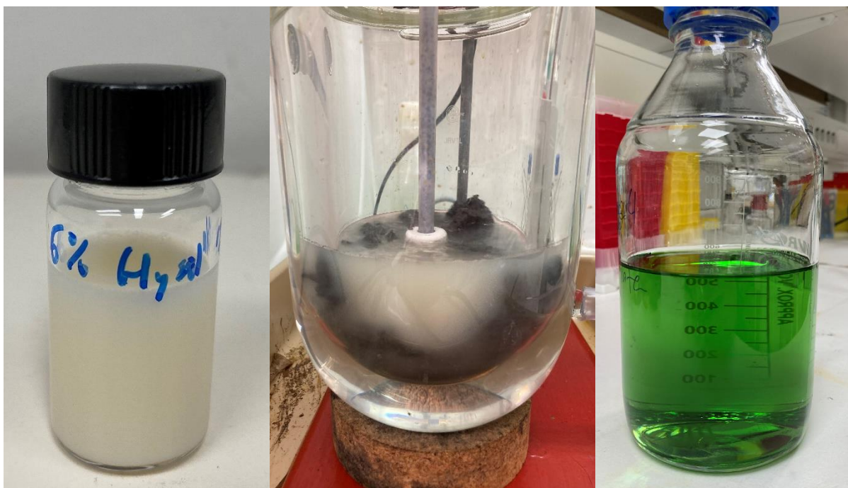
Figure 16: Hysol SL 35 XBB (6%) in water (left), swarf B mixed with water (centre) and filtered leachate (right).
