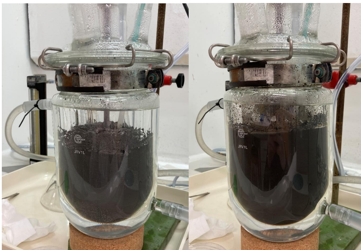
Figure 18: Leaching slurry after 60-90 minutes with a swarf foam on the liquid surface (left), and 180 minutes after disintegration of the cake (right).
