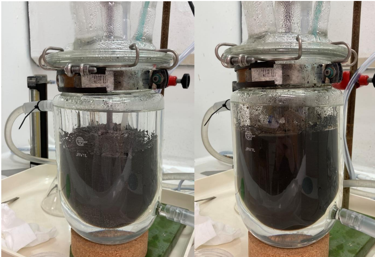
Figure 18: Leaching slurry after 60-90 minutes with a swarf foam on the liquid surface (left), and 180 minutes after disintegration of the cake (right).
