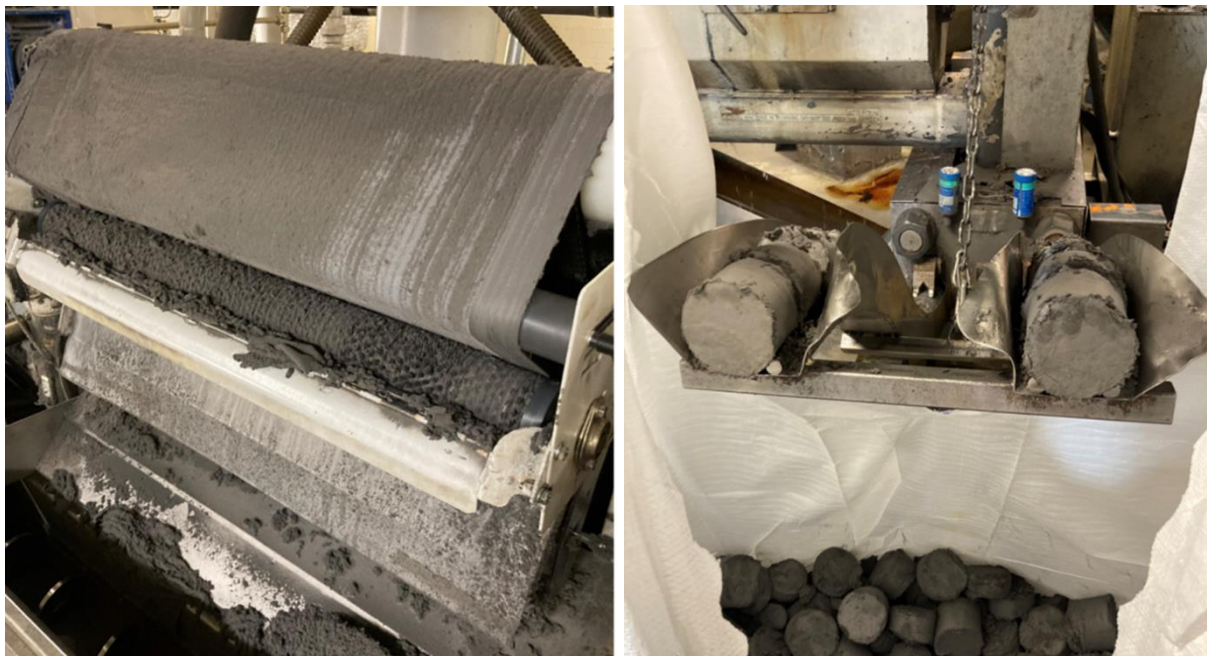
Figure 3: Vacuum filtration (left) and briquetting of grinding swarf (right).
