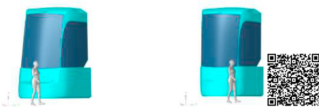
Fig. 3. Generic tram model in compliance with TR17420 with VIVA+ 50F at 15% tram width (left) and steeper front shape at 50% tram width (right) and the QR code of Siemens "Assisted and Driverless Train Operation".
