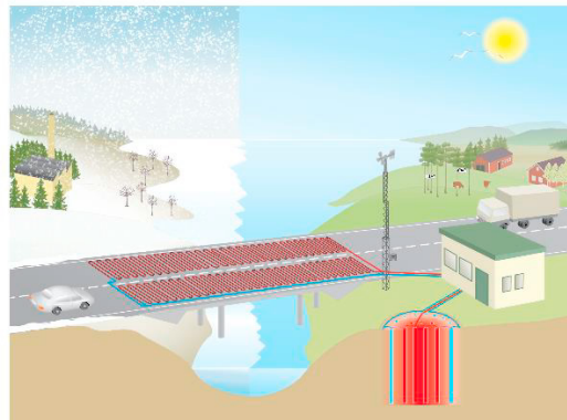
Fig. 1. A hydronic system, utilizing pavement as solar energy collector and seasonal storage by boreholes (Karin Holmgren)
