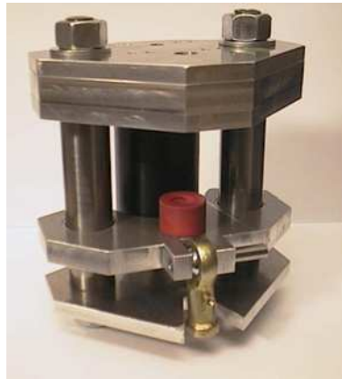
Figure 2: The knee actuator showing the motor in the background and the moving plate in the foreground. The gearbox is hidden inside the top housing.
