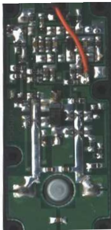
Figure 4: Wire soldered to the servo PCB for sampling of the position signal.
