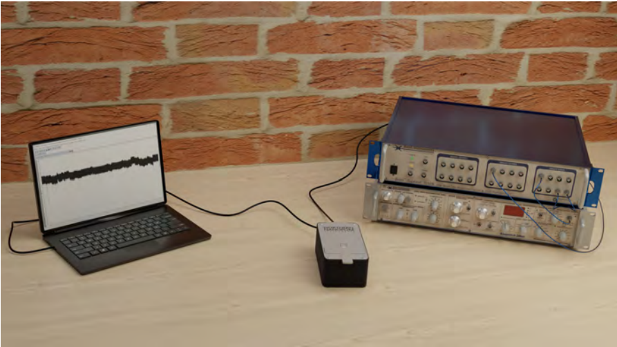
Figure 4.5: The experimental setup for ion current measurements, with the flow cell placed inside the Faraday cage, which is connected to the Axopatch 200B patch-clamp amplifier and the Digidata 1550B digitiser.
