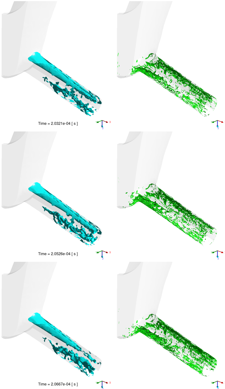
Figure 4.35: Vapor formations ( \alpha = 0.5 ) and turbulent structures ( \lambda_2 = 5 \times 10^{13} ) t4, t5, t6 - TS Model, high lift, LES
