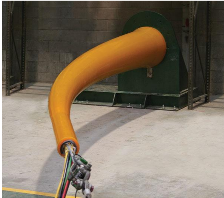
Figure 9: Typical Bending Stiffener Used by Balmoral Offshore[72]
