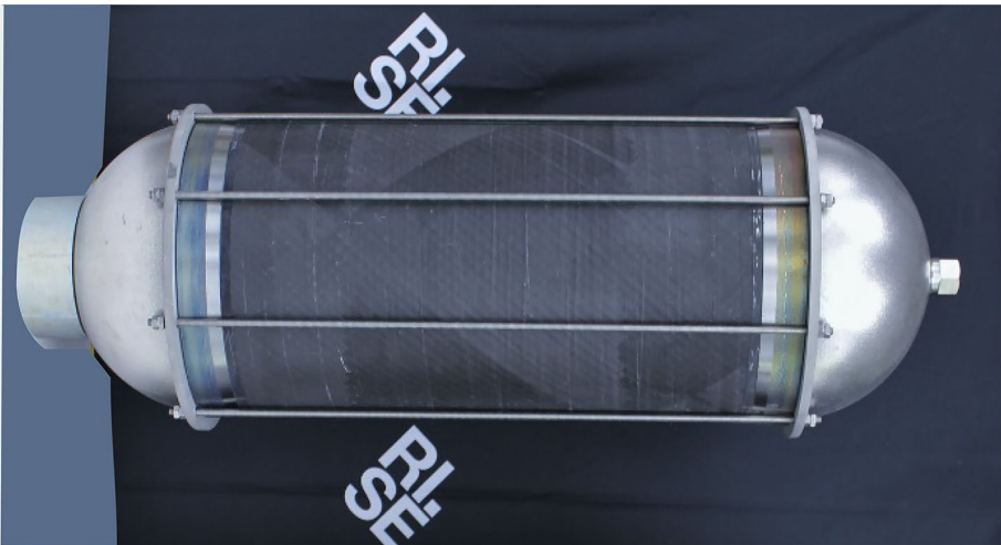
Fig. 13 Vessel ready for testing, with outer safety cage
