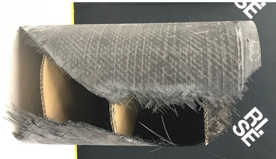
Fig. 19 Fractographic investigation on the debris of the cylinder
