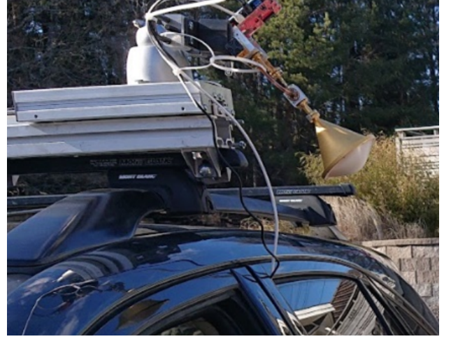
Fig. 3. The radar mounted on a vehicle.
