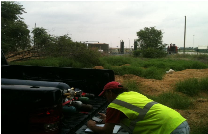
Figure 17 Tracer releases of N_2O from a car upwind of a well and mobile compressor station in Fort Worth.
