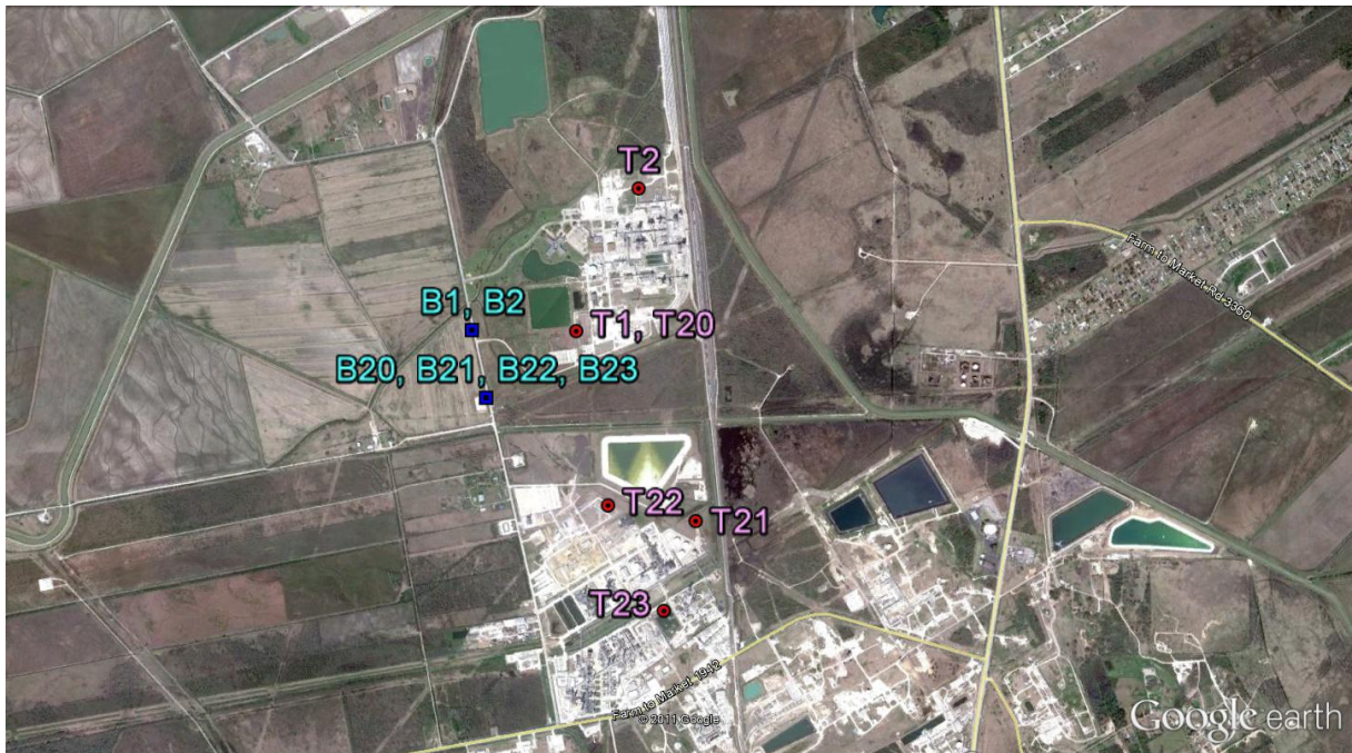
Figure 66 Thermal emission measurement objects around Mont Belvieu (north part). The blue squares indicate the base positions (B) of the infrared telescope, whereas red circles (T) indicate the corresponding thermal emission survey objects. See Table 39 for more detailed information.
