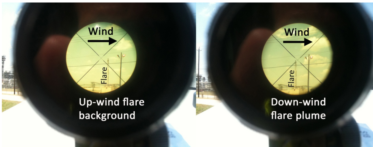
Figure 63 Thermal emission measurements of a flare exhaust plume. The down-wind flare emission signal is subtracted with the up-wind flare thermal background signal. The aiming cross is approximately the centre of the viewing infrared emission telescope.
