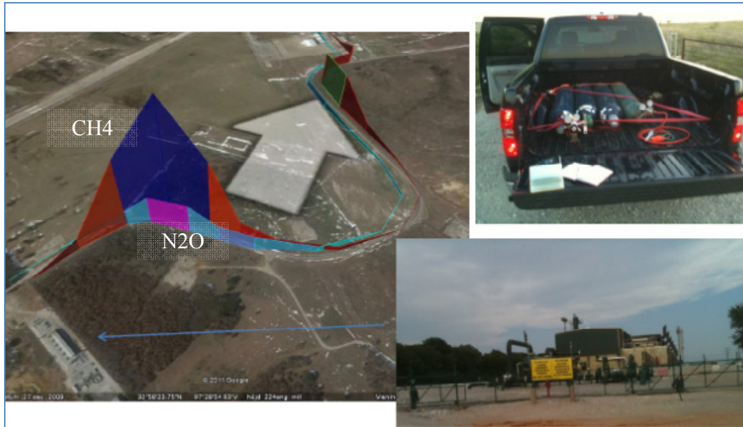
Figure 18 Example of a tracer correlation measurements at a compressor and well pad facility at , 1.8 km SSE of the CAM75 site close to the Kenneth Copeland airfield. The methane (red to blue) and tracer gas (pink to cyan) is shown downwind.
