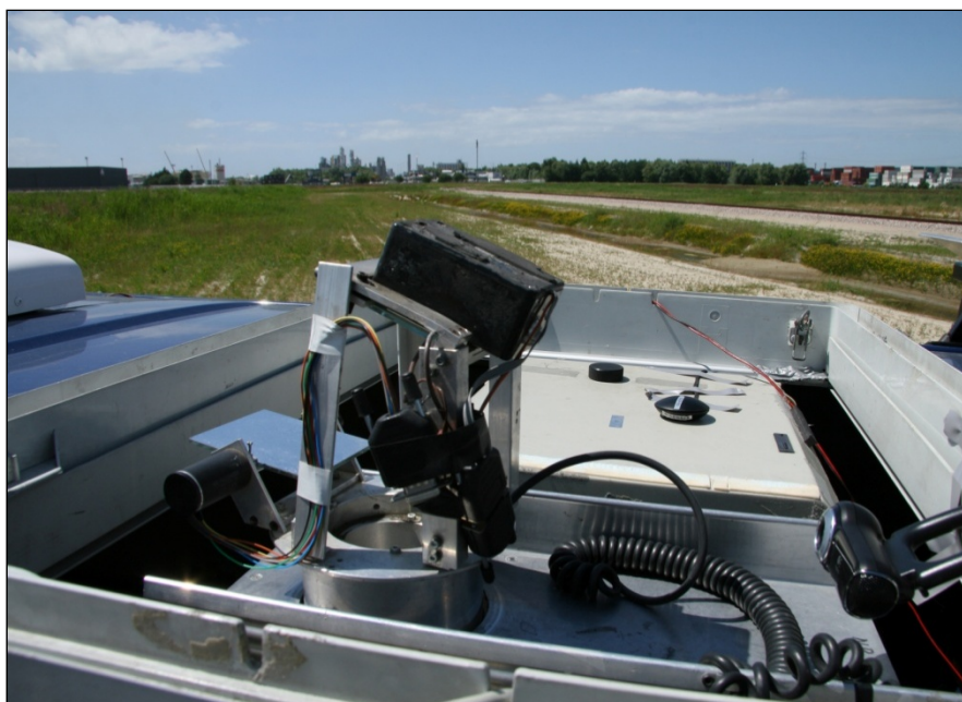
Figure 5 The SOF system elevated through the roof top of the mobile van. The solar tracker (front left) transmits the solar light into the infrared spectrometer (mid right with a GPS on top) independent of the vehicle's position.
