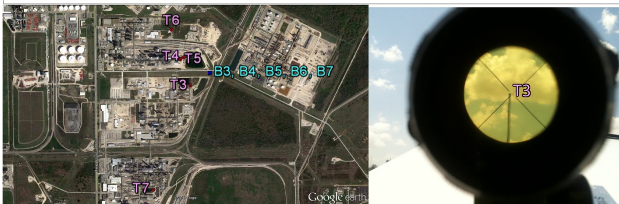
Figure 69 Thermal emission signal acquired at flare T3 around Miller Cut Off Rd in the Battleground area (HSC). The blue squares indicate the base positions (B) of the infrared telescope, whereas red circles (T) indicate the corresponding thermal emission survey objects. See Table 39 for more detailed information. Distinct ethene and propene signatures were observed in the exhaust plume, as seen in the upper part of the figure showing the measured thermal emission signal along with the ethene and propene cross section fingerprints. (Wavenumber 1000\text{ cm}^{-1} corresponds to wavelength 10\text{ }\mu\text{m} ). The aiming scope view (mounted on top of the FTIR) is seen down right.
