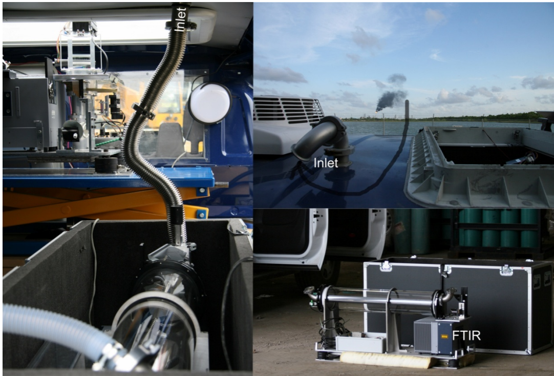
Figure 16 The MeFTIR instrument used in parallel with the SOF system during the campaign. The gas is extracted into the White-cell where it is analysed by infrared absorption measurements. The residence time in the gas cell, and hence the measurements time resolution, is a few seconds.
