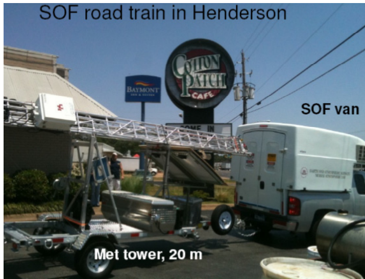
Figure 2 The SOF van and the meteorological tower.
