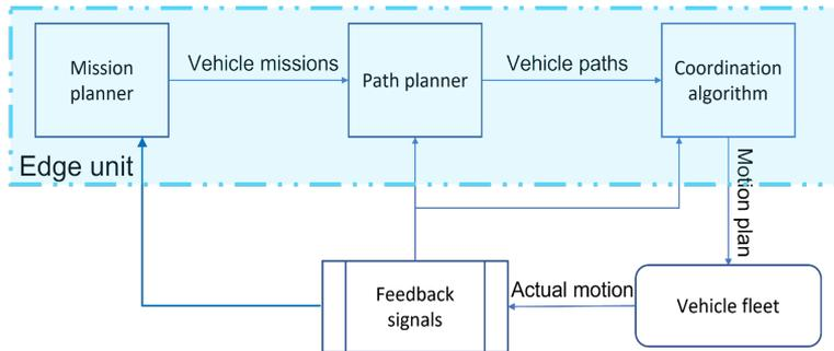
**Figure 1.1:** Architecture of the confined site AV system.
