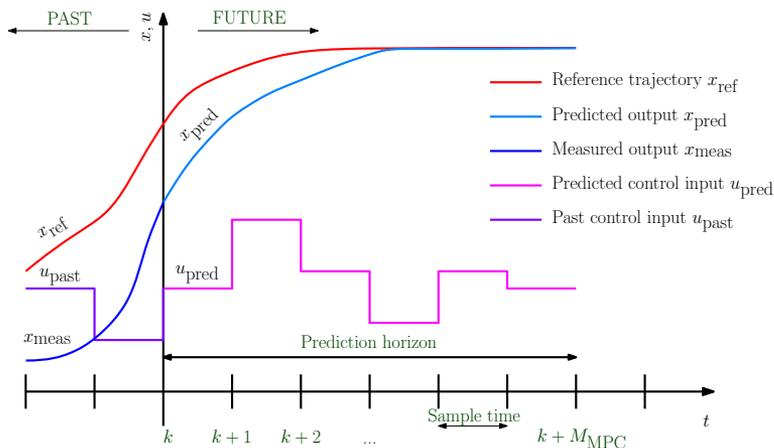
**Figure 2.1:** Illustration of the receding horizon principle.
