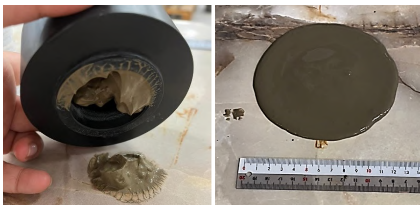
(a) Stiffer mix as observed with mixed clay (b) Improved flows observed with controlled clay particle sizes
