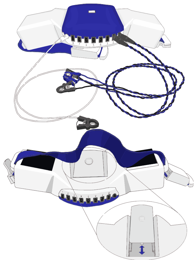
Fig. 2. Design of the MiSMT device. The 8 bipolar electrode jacks are situated on the front of the device. Two of the eight electrode leads, and the reference lead, are drawn. The tactile displays are placed on either side of the device. The battery can be accessed from the bottom.
