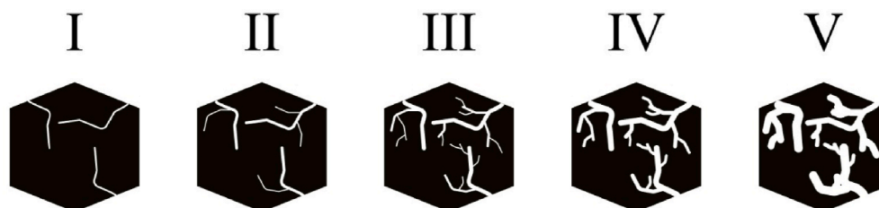
Fig. 3. The variation of pore structure formation through chemical activation in activated carbon. (A colour version of this figure can be viewed online.)
