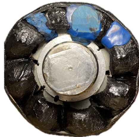
Fig. 9. Image of the prototype rotor postapplication of epoxy resin, fiberglass bandage, and extra material for balancing.
