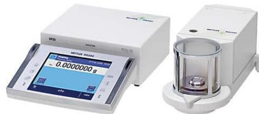
Figure 4.4: METTLER TOLEDO XP6 scale used for the mass gain measurements.
