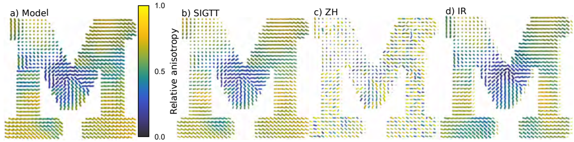
Figure 5.4: Comparison of virtual slices of “M”. a) Virtual slice of simulated sample “M”. b) SIGTT reconstruction. c) ZH reconstruction. d) IR reconstruction. The glyphs are colored according to the relative anisotropy, Eq. (5.2), and scaled according to the spherical mean of each RSM. All three reconstructions follow the orientations of the model reasonably well on average. The SIGTT reconstruction follows both the orientations and relative anisotropy of the model closely. The ZH reconstruction has a lot of variation in the relative anisotropy, as well as many orientations deviating from the overall tendency to follow the model. The IR reconstruction follows the model almost as well as the SIGTT reconstruction.
