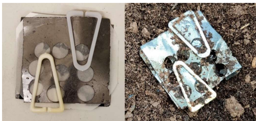
Figure 52. a 5 x 5 cm HSC (left) before and (right) after the biodegradability test. [II]
