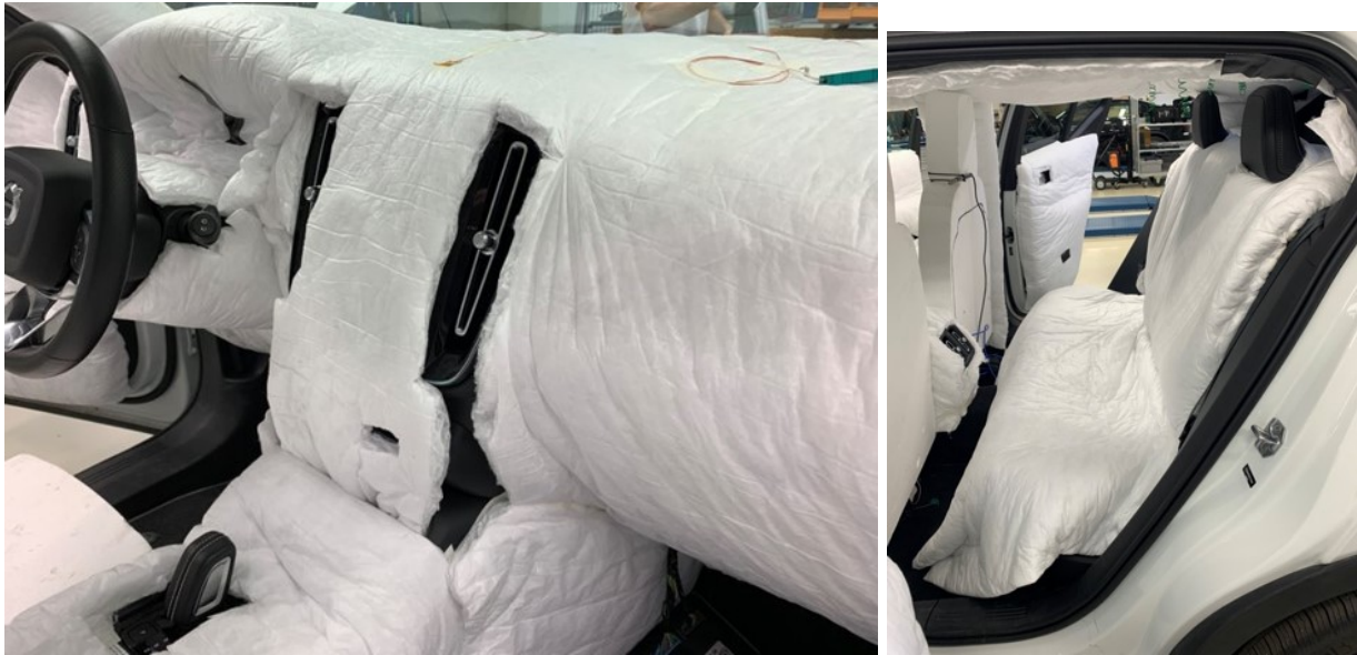
Figure 3.12: Experimental setup of the fully insulated cabin.
