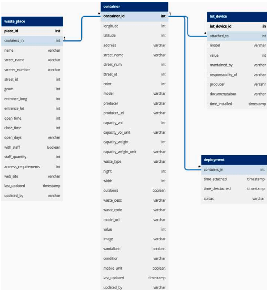
Fig. 5.. Relational data model schema for containers.
