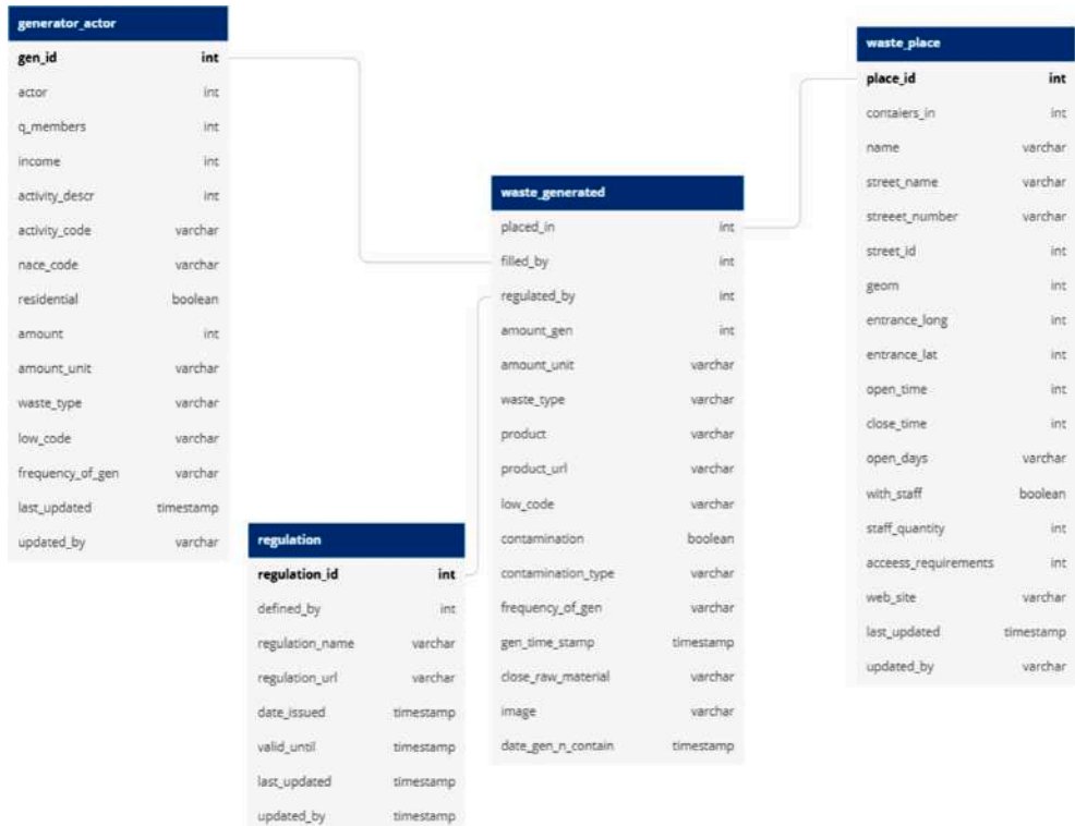
Fig. 12.. Relational data model schema for waste transfers.
