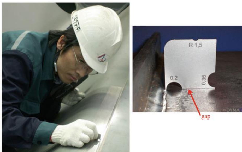
Figure 8: Simple gauge for measuring the depth of the HFMI-groove.
