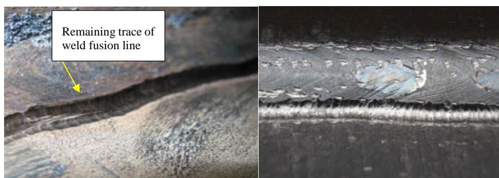
Figure 9: Examples of properly and improperly treated welds. The left image includes a trace of the weld fusion line remaining in the HFMI-groove which is unacceptable. The HFMI-groove in the right image is defect-free with a smooth and shiny surface.
