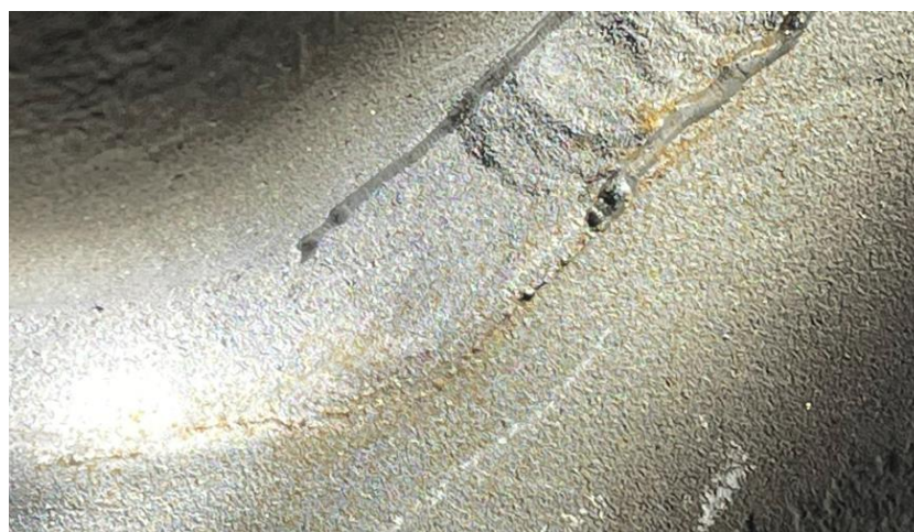
Figure 10: HFMI treatment revealing shallow, sub-surface porosity. Also visible are surface (possibly cold) cracks at weld toe. Such weld should be repaired and re-treated.
