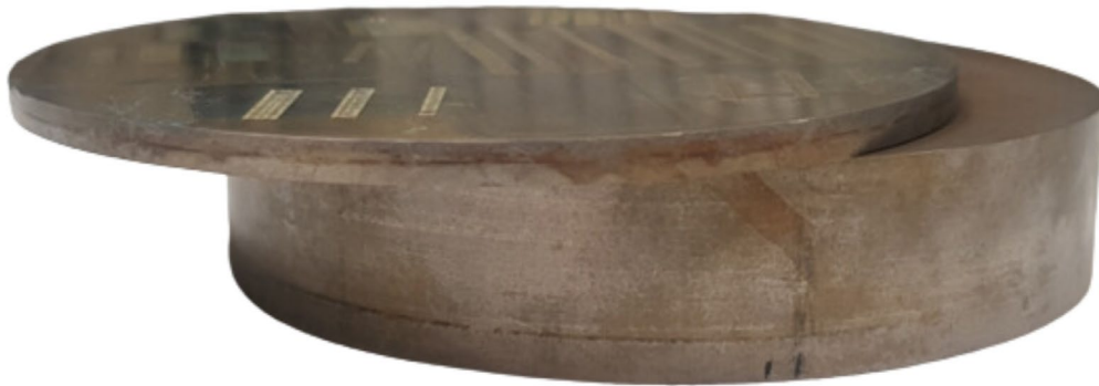
Figure 16: slice cut from build plate surface to prepare samples for microscopy
