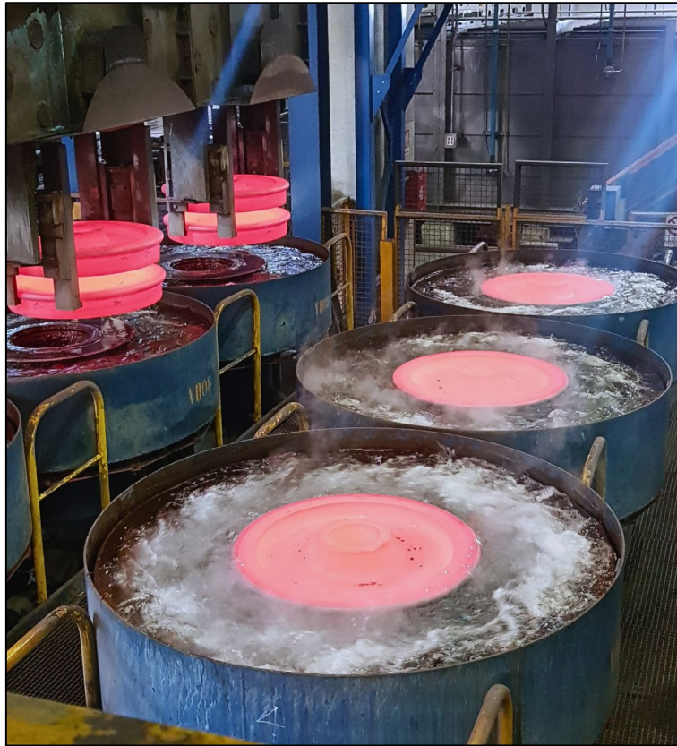
Figure 5: Rim chilling facilities at Lucchini RS in Lovere, Italy
