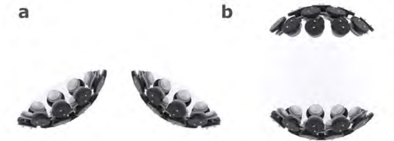
Figure 3.1: Array configurations of an acoustic levitator of a) single-side independent arrays, and b) coupled arrays forming a cavity.
