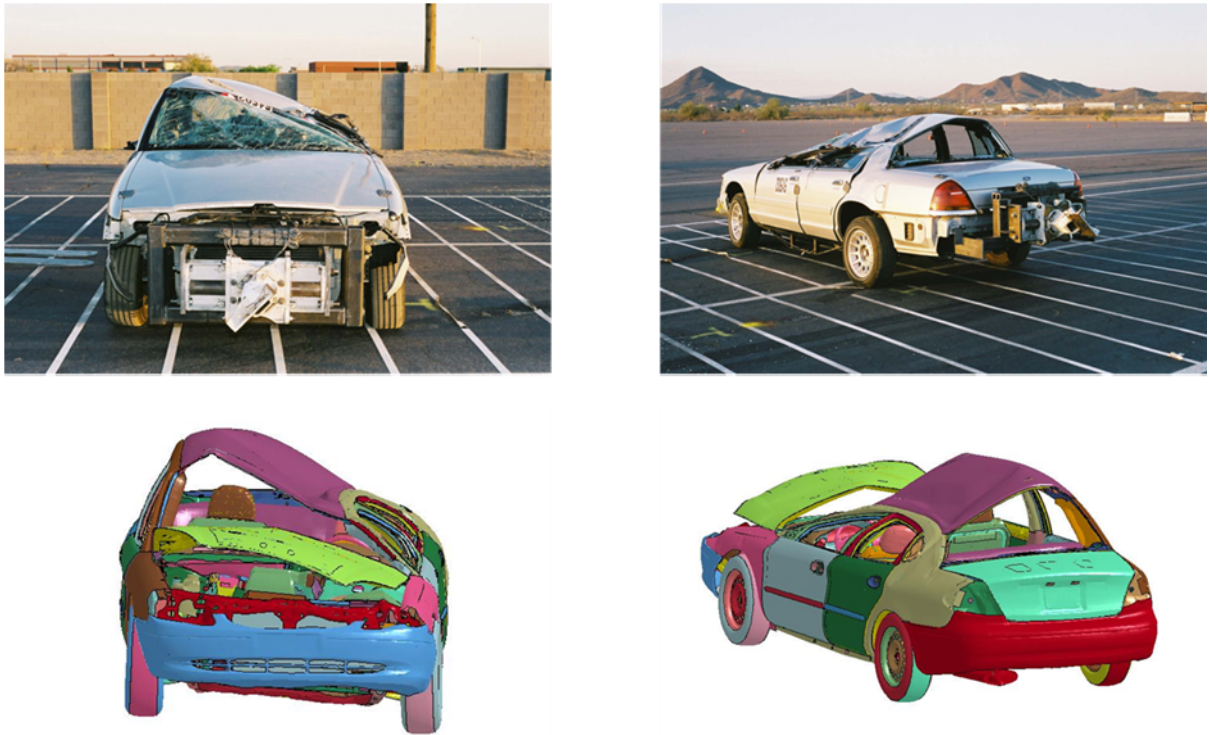
Fig.3.7. Qualitative crush comparison of production Crown Victoria (top) from test 51502 and modified Taurus model (bottom) subjected to same input conditions adjusted for same touchdown location.
