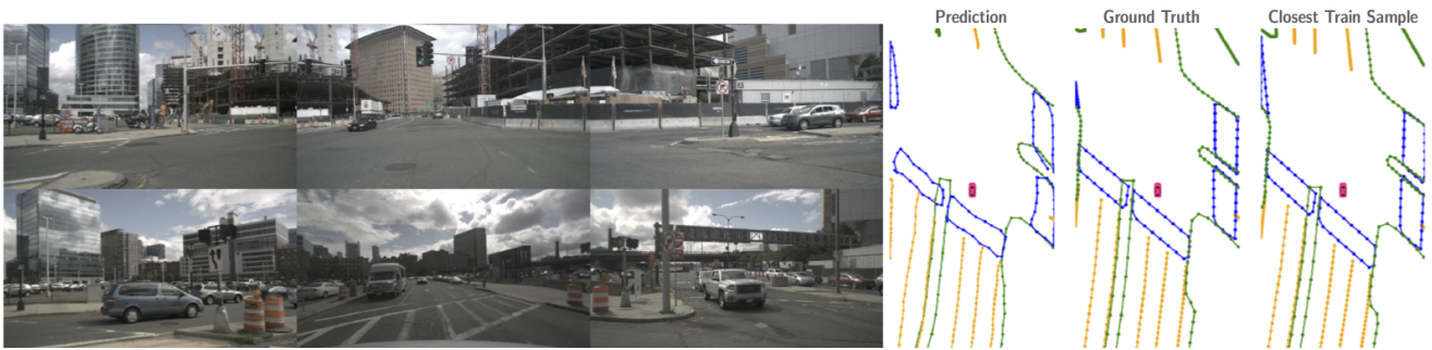
Figure 2. Example from nuScenes where input images, predictions, and ground truth for a test sample are displayed together with the ground truth of the closest train sample. Lane dividers, road boundaries, and pedestrian crossings are visualized in orange, green, and blue.
