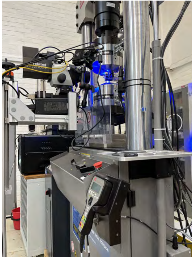
Figure 3.11: Stereo microscope set up for crack measurement and DIC measurement in Paper C
