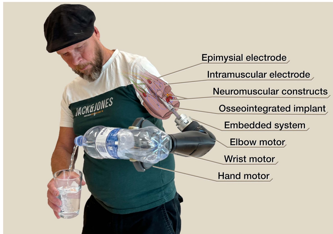
Figure 1. Detail overview of the neuromusculoskeletal prosthesis. Shown are electrodes on native muscles and in native muscles as well as free muscle grafts reinnervated by the median, radial, and ulnar nerve (i.e. electro-neuromuscular constructs). Furthermore, the attachment mechanism, where a clamp mechanism connects the prosthesis to the percutaneous part of the osseointegrated titanium implant is shown. Beneath the clamp, a housing with the embedded system is situated which decodes and translates motion intent to actuate the hand, wrist, and elbow motors of the prosthesis. Overlay surgical illustration repurposed from [28]. Adapted with permission from AAAS.
