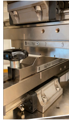
Figure 2: Fixture for ZD-tests.
