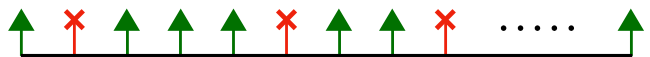
Fig. 1: Illustration of a sparsely distorted linear array, where the red crosses denote distorted sensors.
