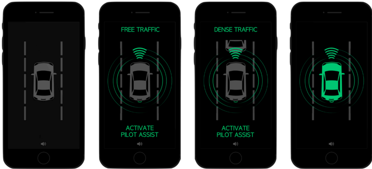
Fig. 1a. Front-end design for Driver Coach app (from left to right: PA_off status, Recommendation event – Sparse traffic, Recommendation event – Dense traffic, PA_on status).
