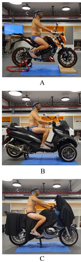
Figure 1. Measuring process of a volunteer positioned on the three PTWs: naked (A), scooter (B), and touring (C).
