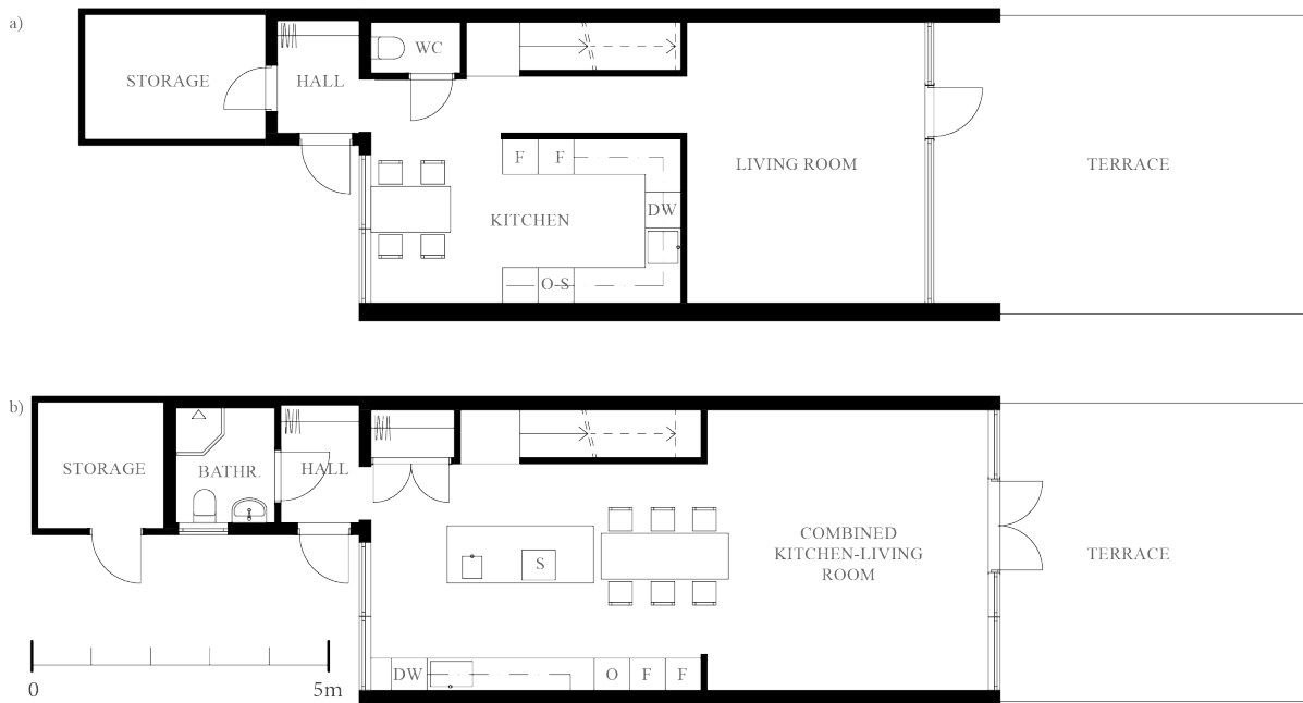
Figure 6 – The floorplan of the terraced house (I-3) before (a) and after (b) the alterations (DW: dishwasher, F: fridge or freezer, O: oven, S: stove) (as published in Paper B)
