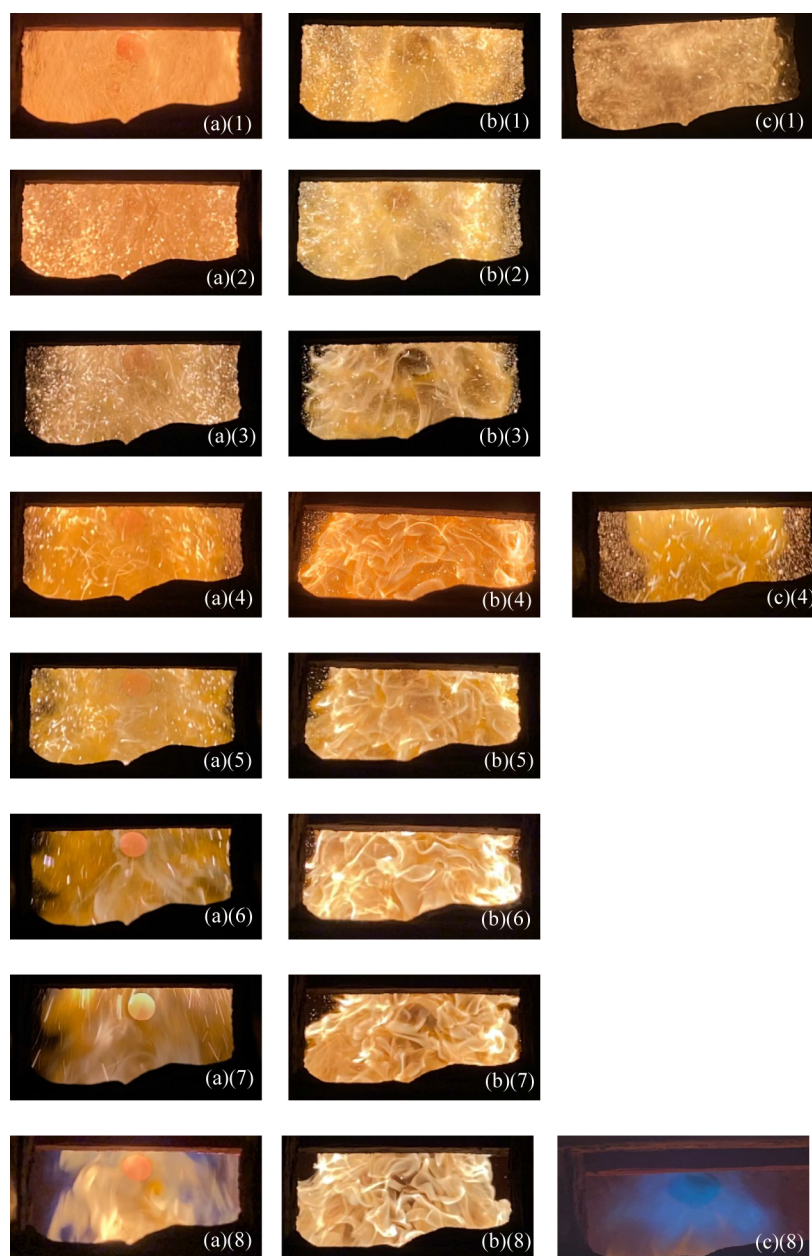
Figure 4. Photographs taken at M2: (a) \lambda 1.15, 70 l/min transport air; (b) \lambda 1.623, 70 l/min transport air; (c) \lambda 1.15, 130 l/min transport air—only three cases are presented for these settings. The following cases were studied: (1) 100% lignite; (2) 10% propane, 90% lignite; (3) 30% propane, 70% lignite; (4) 50% propane, 50% lignite; (5) 70% propane, 30% lignite; (6) 90% propane, 10% lignite; (7) 95% propane, 5% lignite; and (8) 100% propane.
