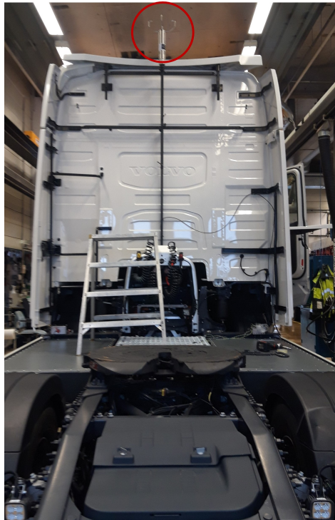
Figure 3. The test vehicle with an anemometer on the cab roof.
