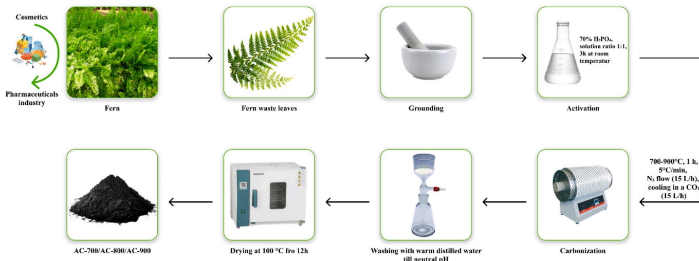
Fig. 1. Schematic preparation procedure of activated carbons.
