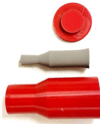
Punch moulds with 5 mm thickness
