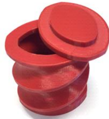
Screw mould with 10 mm thickness
