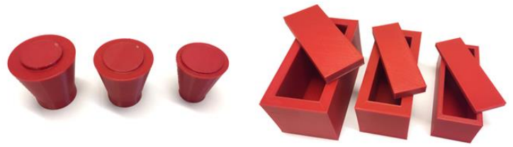
Cone mould with different thicknesses of 10mm, 7.5 mm & 5mm
