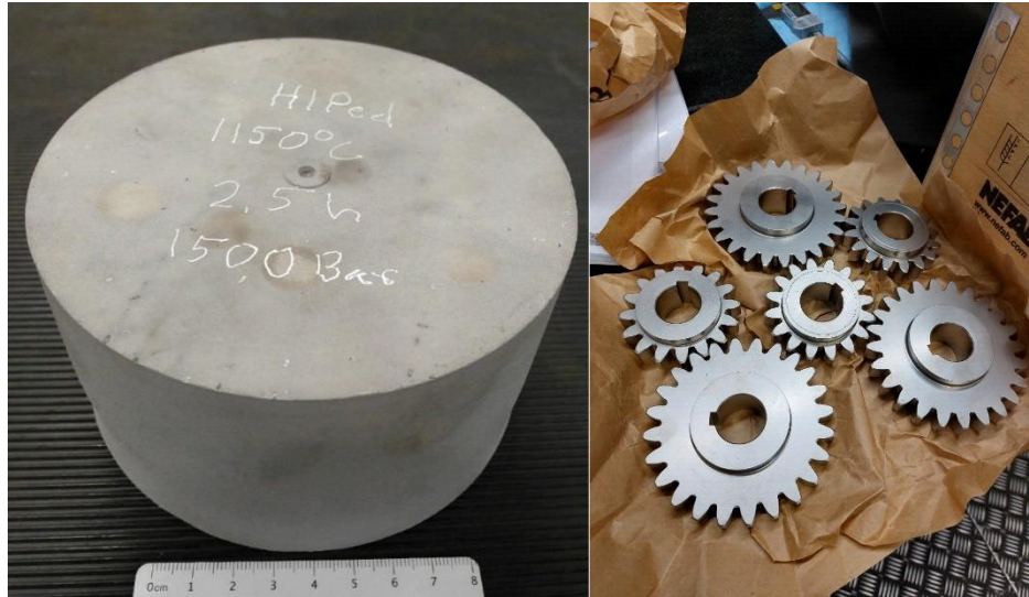
Figure 15.(a) Cylindrical puck of high-performance PM steels fabricated through cold isostatic pressing (CIP), high temperature sintering (1250 °C) and capsule-free hot isostatic pressing (HIP) processes (b) gears machined from this puck.
