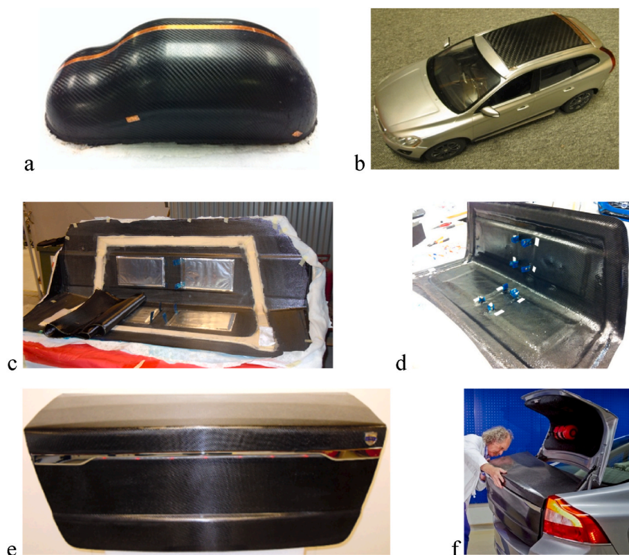
Fig. 1. (a,b) Desktop scale (approximately 30 cm long) structural supercapacitor composite demonstrators in the form of automotive exterior panels able to power lights [9], (c–f) Full scale Volvo S80 boot lid demonstrator with integrated structural supercapacitors to power external lights [9].
