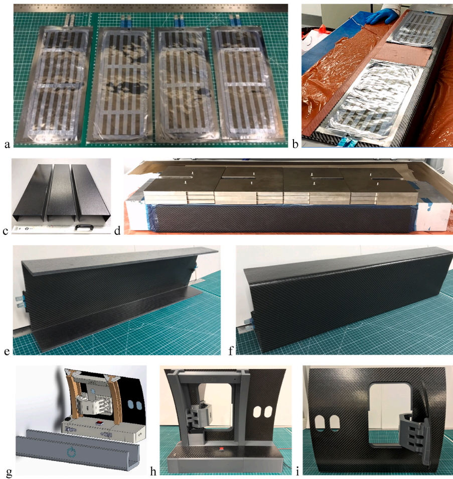
Fig. 6. (a) Four of the twelve structural supercapacitor composite cells, (b) cells integrated into the beam, (c) inner, central and outer structural shells, (d) consolidation and curing of the SPC beam, (e) inner surface of the SPC beam, (f) outer surface of the SPC beam, (g) computer aided design model of scaled fuselage door assembly and SPC beam, (h) inside and (i) outside of fuselage door assembly. For an indication of scale, the cells are 30 cm long, the beam is 80 cm long and the fuselage is 40 cm wide.
