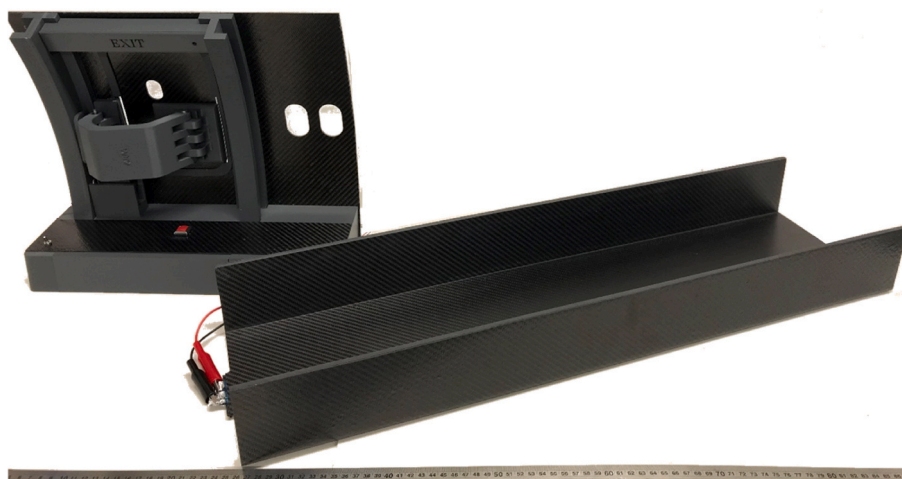
Fig. 13. Multifunctional fuselage beam demonstrator electrically connected to aircraft door model.
