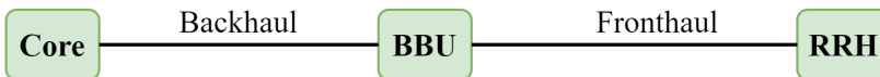
Figure 2.1: Network structure for 4G including: core, backhaul, baseband unit (BBU), fronthaul and remote radio head (RRH).
