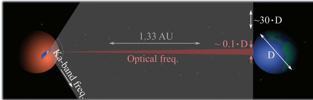
Figure 1.2: Beam divergence for a 32 GHz RF-beam with 3 m diameter transmitter and a 193.5 THz optical beam with a 10 cm diameter transmitter.
