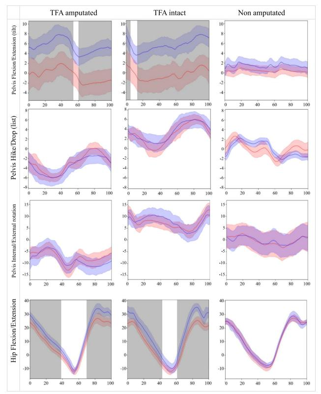
Fig. 2 Joint angles averaged over all gait cycles. Blue = Inertial motion capture system  $\pm$  IQR. Red = Optoelectronic system  $\pm$  IQR. Shaded bands show regions where median RMSE > 5°. Gait cycle (%) horizontal axis is plotted against joint angles (°) on the vertical axis
