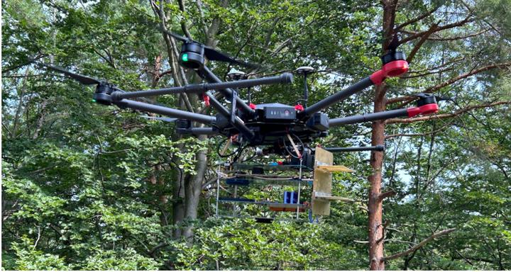
Figure 3.1: **Transmitter Unit** Picture of the L-band transmitter unit mounted underneath a hovering UAV. A schematic of the transmitter is shown in Fig. 3.2
