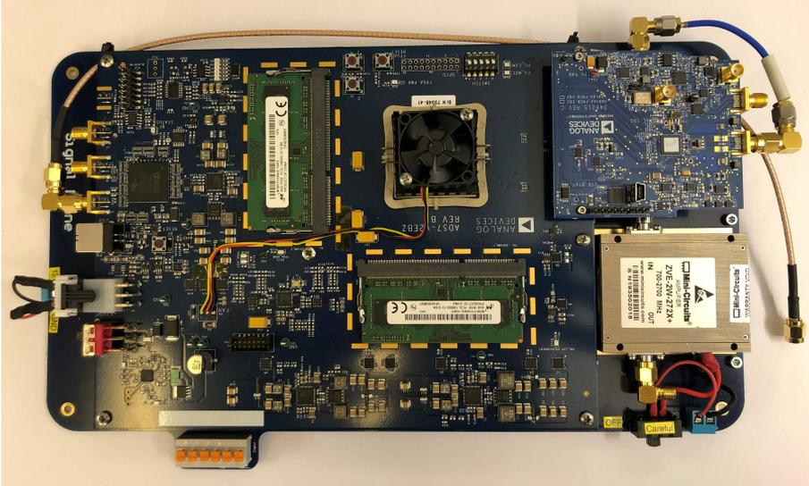
Figure 3.3: **Waveform Generation Plane** A picture of the waveform generation plane described in Section 3.1.1. The plane consists of an FPGA, a DAC, a class-A amplifier, a band-pass filter (located underneath the DAC), and connectors and switches. The dimension of the PCB to which the components are mounted is  $315 \times 175$  mm.
