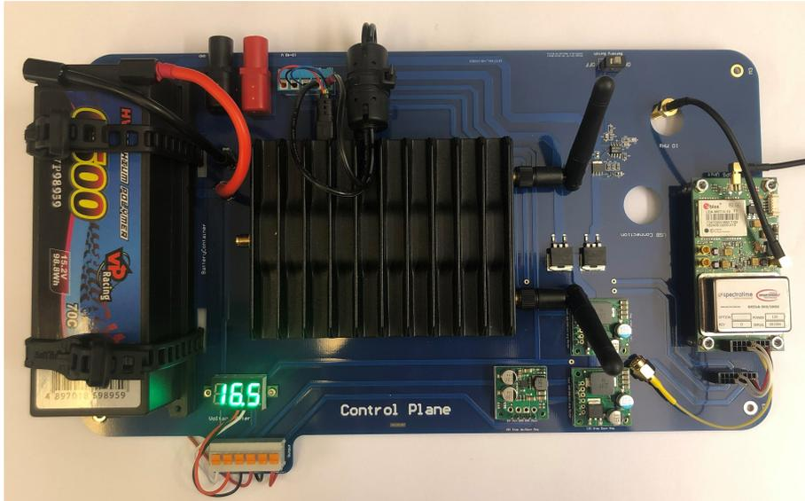
Figure 3.4: **Control Plane** A picture of the control plane described in Section 3.1.2. The plane consists of a mini-computer, a LIPO battery, a GNSS unit, and various electronic components. The dimension of the PCB to which the components are mounted is  $315 \times 175$  mm.
