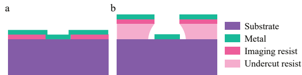
Figure 4.10: Lift-off with two different resist profiles. a A too thin resist without an undercut results in a continuous layer of metal on the sidewall, preventing lift-off. b A thicker resist stack with an undercut profile in the bottom resist facilitates liftoff. In our stack we use PMMA as the imaging layer, with MMA underneath. As MMA is more soluble in developer than PMMA, it will develop faster than the exposed PMMA, creating an undercut.
