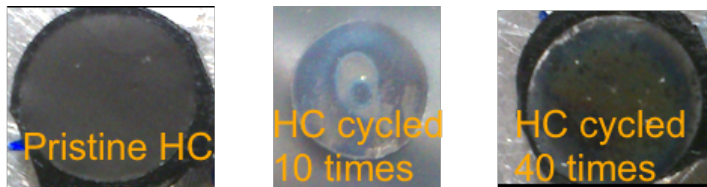
Figure 3.10: Hard carbon electrodes before and after cycling.
