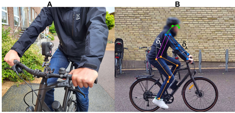
Figure 1. Panel A: Camera mounted on bike, Panel B: estimated posture and angles
