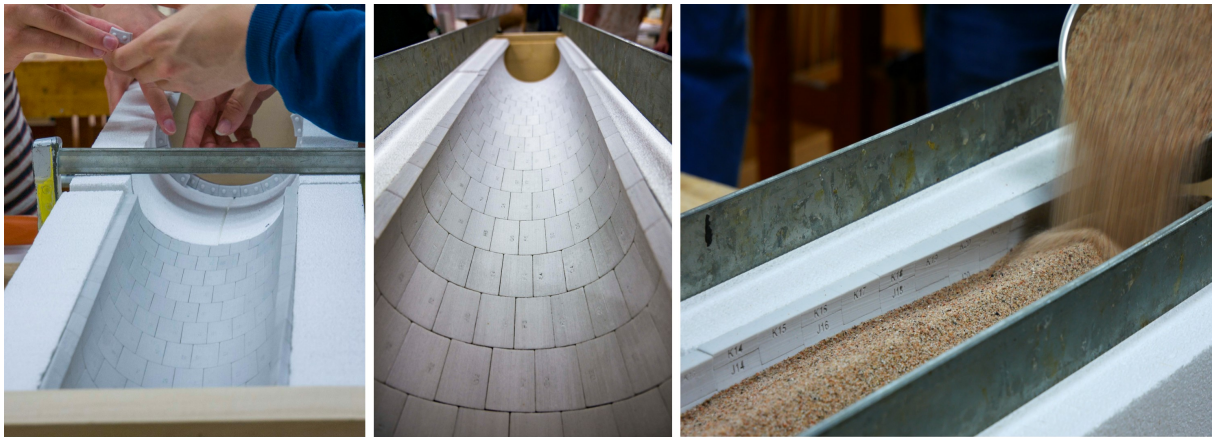
Figure 6: The construction process of a model bridge. Left, the 3D printed blocks are assembled without glue. Rounded extrusions are for easier assembly but do not contribute to any bending stiffness. The middle shows the bridge before filling it with sand as in the right image.
