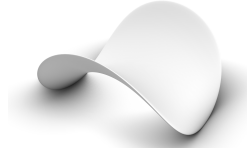
(c) A shell structure in the form of Enneper's minimal surface
