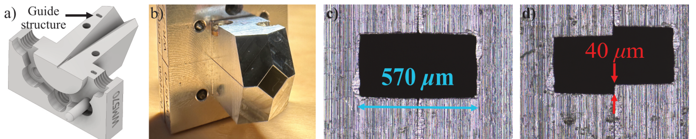
Fig. 4: WM570 diagonal horn antenna. a) CAD model of the antenna. b) Photograph of the machined horn antenna in Aluminum E-plane split-blocks. c) Micrograph of WM570 waveguide aperture when aligned. d) Micrograph of WM570 waveguide aperture with 40\text{-}\mu\text{m} misalignment.
