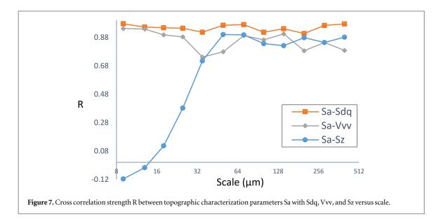
wavelengths from 9 to  $400 \,\mu\text{m}$ . The bandpass filter is described above. For simplicity, the factor of four is omitted in the calculations here. This omission does not affect the correlation strengths; it simply shifts the parameter values on the abscissa.
