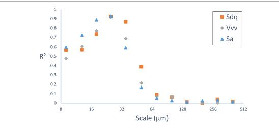
$\label{eq:Figure 6.} Feasults of multiscale regression analyses showing coefficients of determination (R^2) of friction with Sdq, Vvv, and Sa versus scale.$
